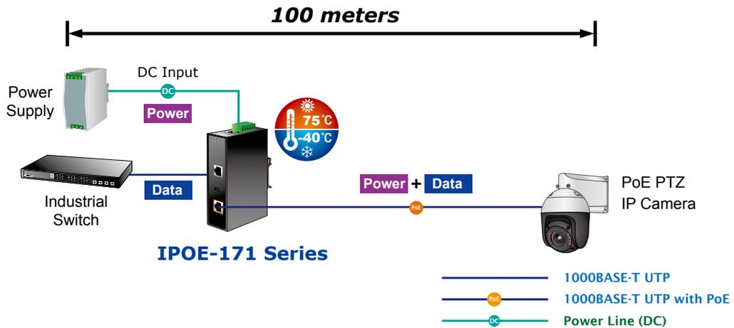
*Installation of 802.3bt PoE Injector and Splitter*
