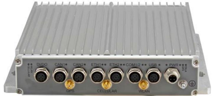
The BC50R is a maintenance-free box computer that has been designed, e.g., for data acquisition applications in rugged environments in vehicles, e.g. in trains, commercial vehicles, mobile machines or ships. All interfaces are implemented on rugged M12 connectors (USB, digital input and output, Gigabit Ethernet, CAN and legacy serial I/O). The housing is compliant to the IP65 protection class.
