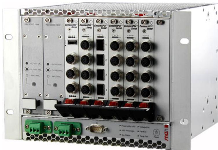
The NH30 is a modular turn-key network switch solution with carrier grade Layer 2 and Layer 3 VLAN routing capabilities offering a seamless throughput of 29 Gbit/s. It is designed for use in trains, trams or industrial environments.
