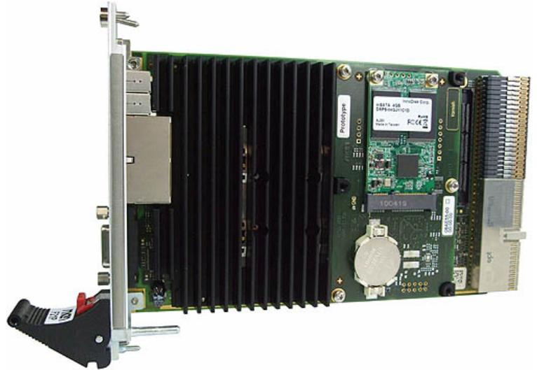
The F23P versatile 3U 4HP single-board computer is a member of the scalable family of Intel® CPU boards which ensures future-safety and long-term availability of a system.
